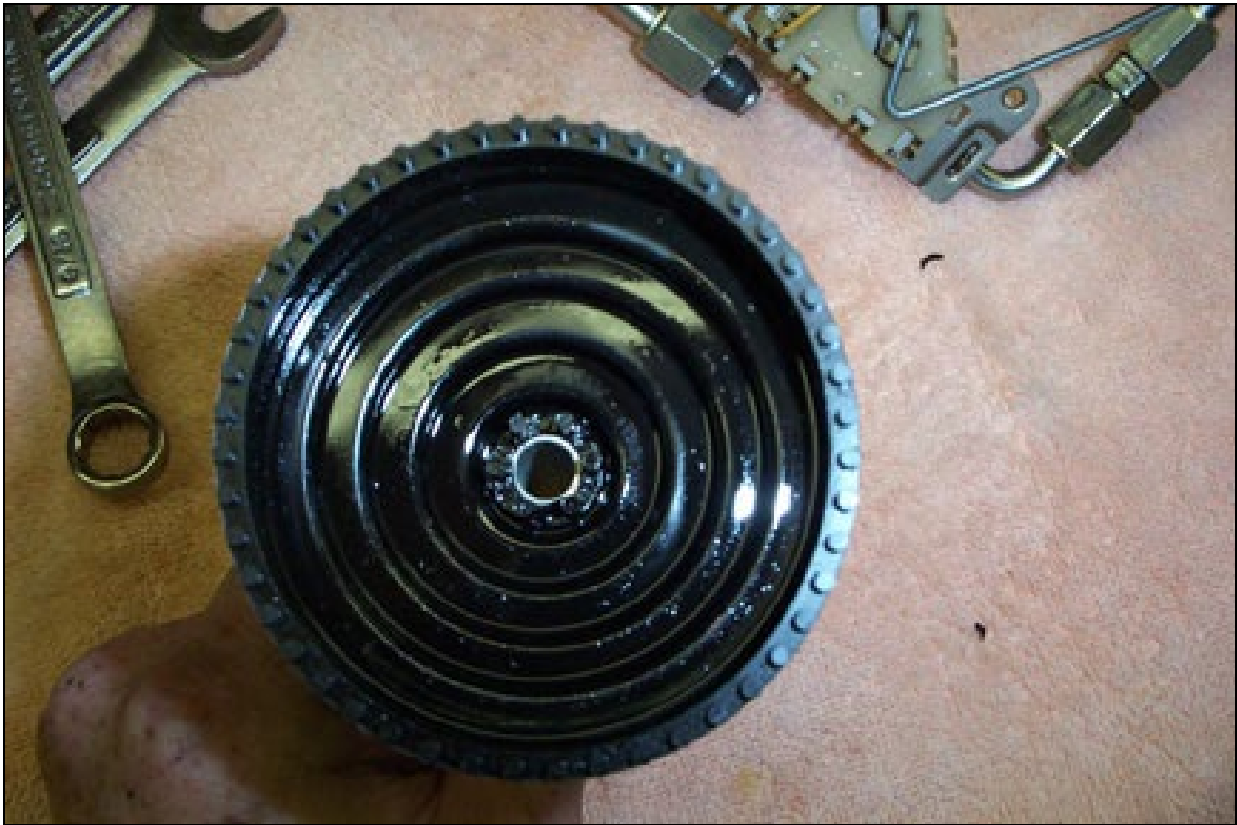
Figure 9 – Pickup Tube Installed in Strainer
