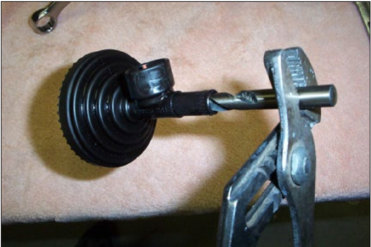
Figure 8 – Clearancing Pickup Strainer for Pickup Tube
